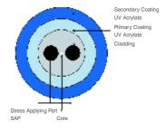
With dual-layer, UV-cured Acrylate coating, YOFC polarization maintaining fibre has high environmental stability performance over the temperature range of  $-45^{\circ}$ C to  $+85^{\circ}$ C ( $-49^{\circ}$ F to  $+185^{\circ}$ F).
